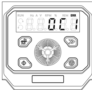
c: Fault status display
